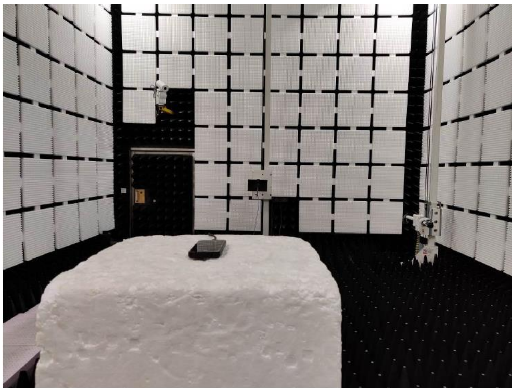
Photo of Radiated emission Measurement (Above 1GHz)
