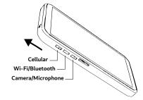
Enable Cellular and Wi-Fi features by pushing those switches up, away from the SIM slot, as shown.
